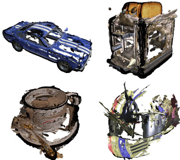
Figure 7. Visualization of the reconstruction results by COLMAP on the ShinyBlender dataset. COLMAP failed to reconstruct objects with reflective surfaces, as the multi-view consistency was not plausible.
